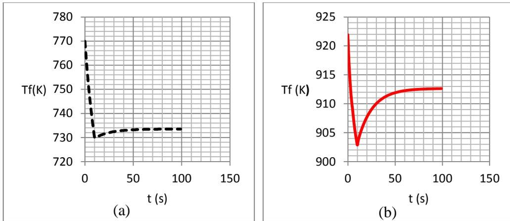
Fig. 4 The graphical analysis of the time evolution of the Overcooling Accident Without Scram (OVC WS) depicting the variation of the (a) Coolant outlet temperature  $T_c$  (K) with time  $t$ (s) (b) Maximum fuel temperature  $T_f$  (K) with time  $t$ (s)
