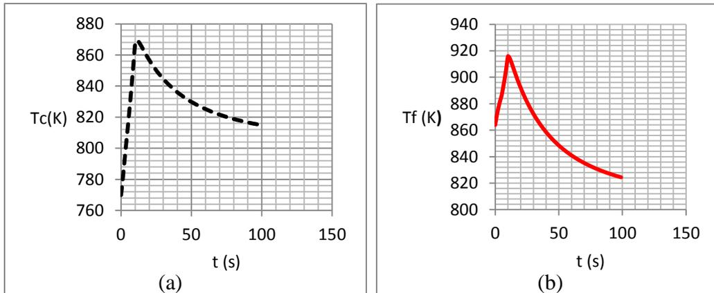
Fig.3 The graphical analysis of the time evolution of the Loss-of-Heat-Sink Without Scram (LOHS WS) depicting the variation of the (a) Coolant outlet temperature  $T_c$  (K) with time  $t$ (s) (b) Maximum fuel temperature  $T_f$  (K) with time  $t$ (s)
