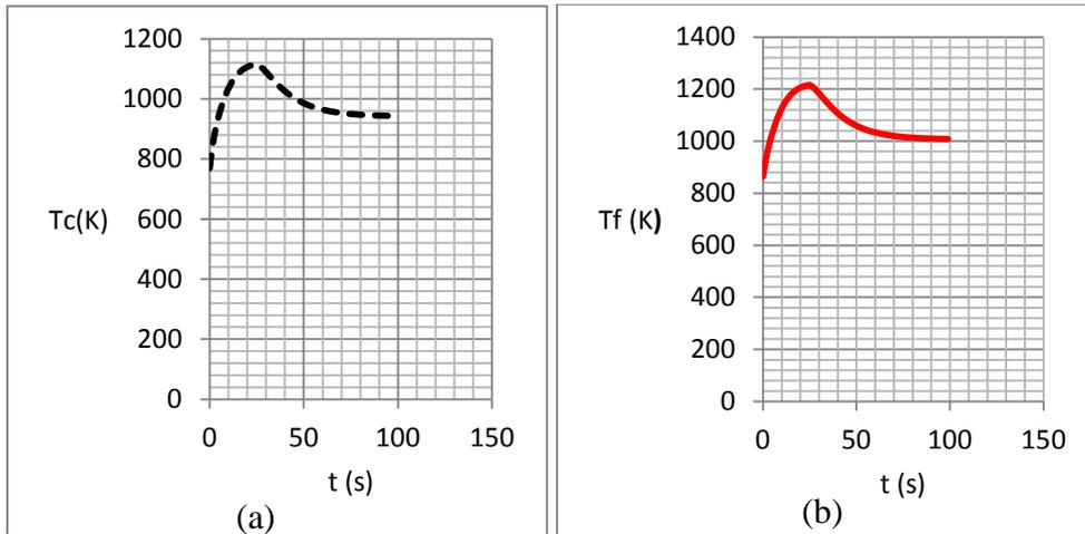
Fig. 1 The graphical analysis of the time evolution of the Loss-of-Flow Without Scram (LOF WS) depicting the variation of the (a) Coolant outlet temperature  $T_c$  (K) with time  $t$ (s) (b) Maximum fuel temperature  $T_f$  (K) with time  $t$ (s)
