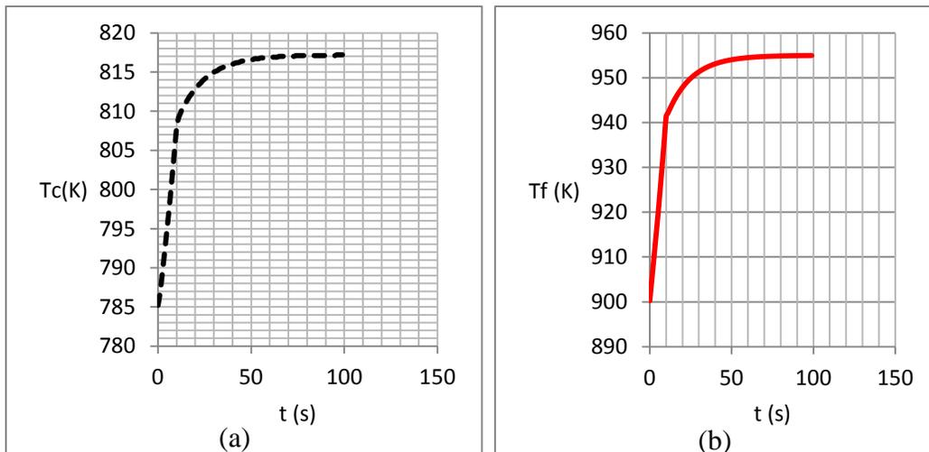
Fig. 2 The graphical analysis of the time evolution of the Transient Overpower Without Scram (TOP WS) depicting the variation of the (a) Coolant outlet temperature  $T_c$  (K) with time  $t$ (s) (b) Maximum fuel temperature  $T_f$  (K) with time  $t$ (s)
