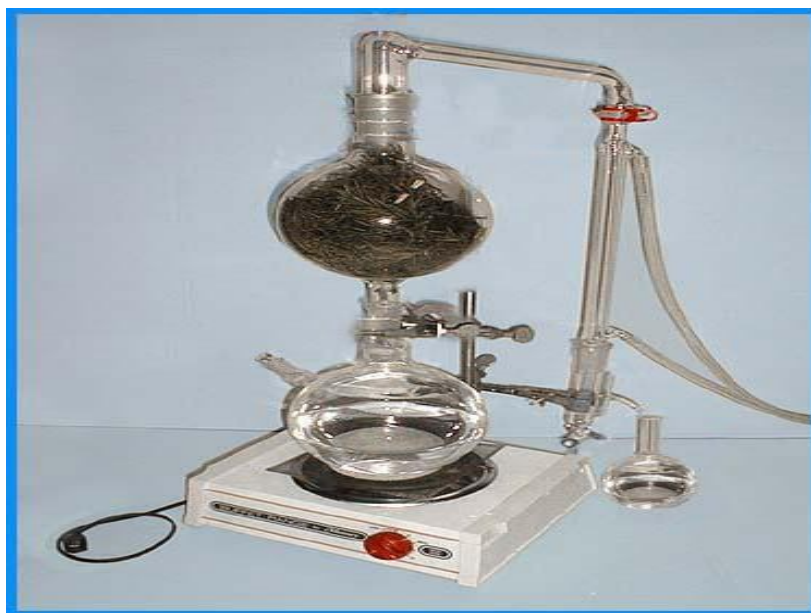
Figure1: Experimental set up for extraction of essential oil from Lemon grass by steam distillation
